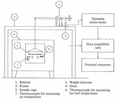
Fig. 3. The experimental device
