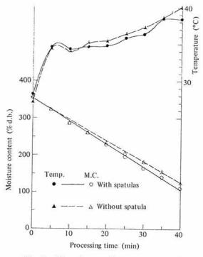
Fig. 8. The change of temperature and moisture content of the leaves in the primary drying process
